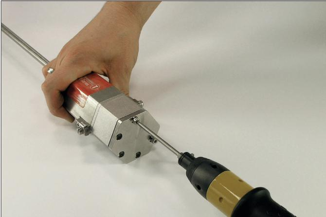
**1** Loosen the five M4×10 screws (A/F 3).
