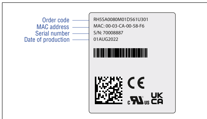
Fig. 1: Example of nameplate of R-Series V RH5 sensor with POWERLINK output
