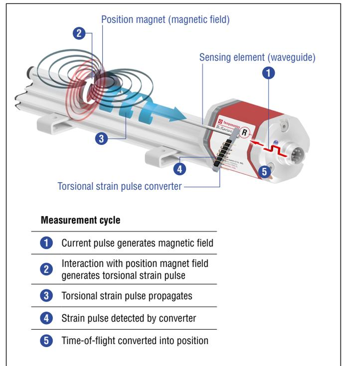
Fig. 2: Time-of-flight based magnetostrictive position sensing principle
