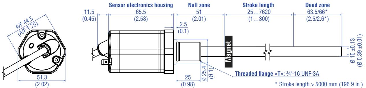
RH5-T-A/F/V – RH5 with threaded flange ¾"-16 UNF-3A with raised-face, example: Connection type HXX/RXX/TXX (straight cable outlet)
