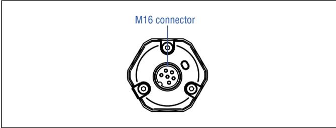
Fig. 74: Location of connection (example M16 connector outlet)
