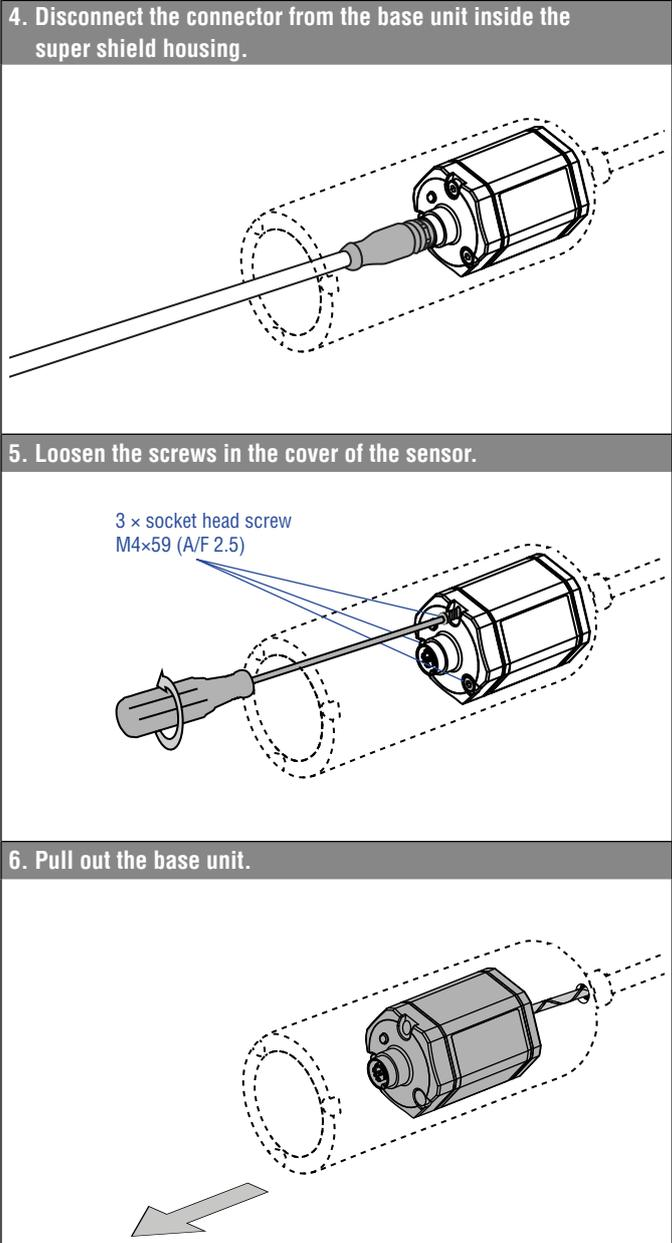
Fig. 69: Replacement of the base unit on model RM5, part 2
