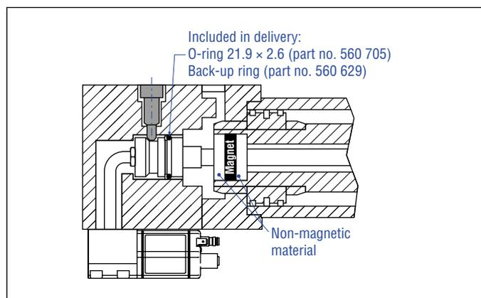
Fig. 45: Mounting example of pressure fit flange »S« and sensor electronics with bottom cable entry
