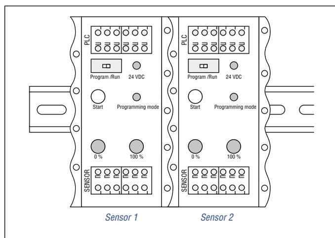
Fig. 104: Installation of cabinet programmer on a 35 mm standard rail
