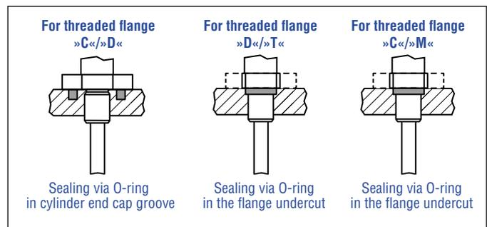
Fig. 41: Possibilities of sealing
