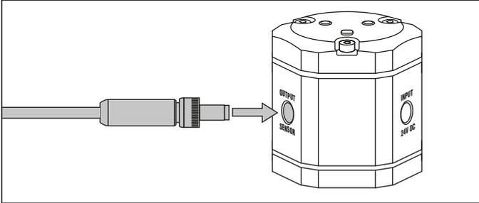
Fig. 84: Connection of adapter cable to TempoLink® smart assistant
