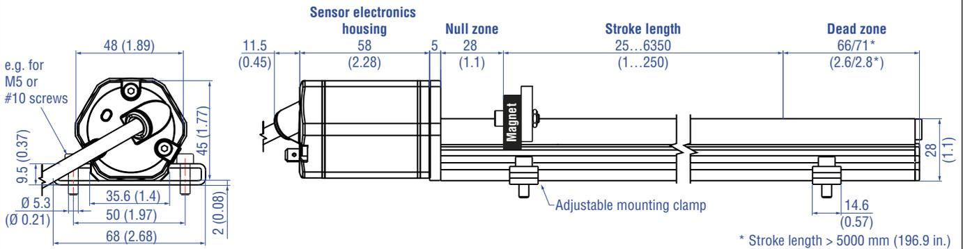
RP5-M, example: Connection type HXX/RXX/TXX (straight cable outlet)
