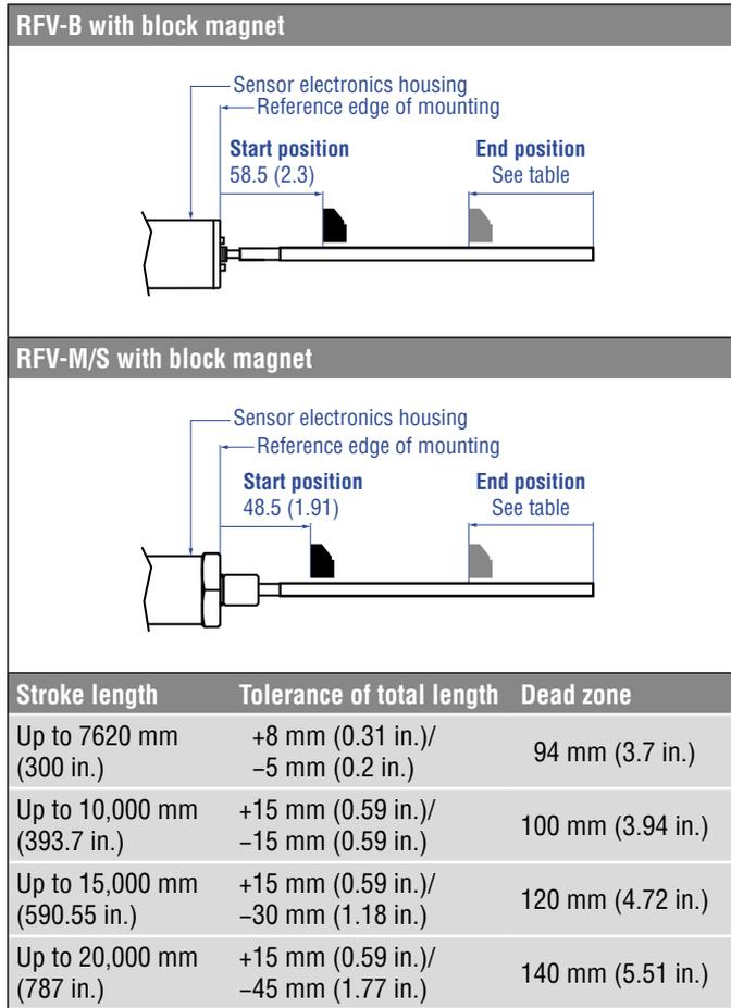
Fig. 58: Start- and end positions of magnets for RFV with block magnet
