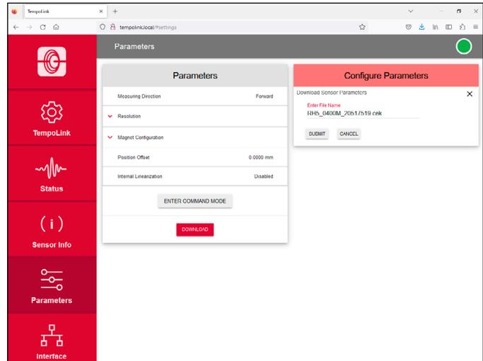
Fig. 97: Download a cek file with the settings of the sensor
