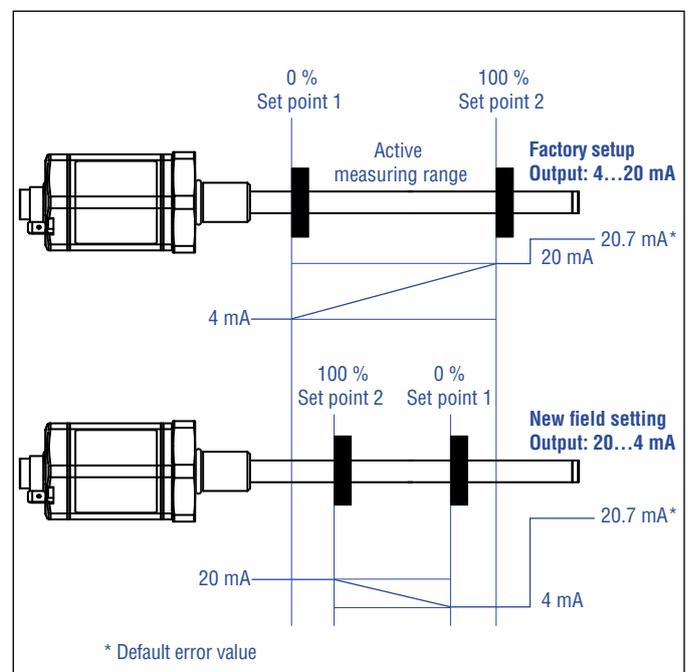
Fig. 83: Reversal of the measuring direction by adjusting the start value (set point 1) and the end value (set point 2)
