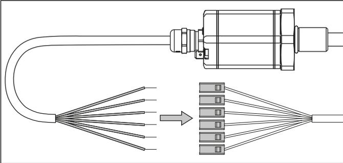
Fig. 87: Connection of adapter cable to R-Series V sensor with cable outlet
