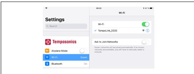
Fig. 92: Choose the network “TempoLink\_XXXX” in the Wi-Fi settings of the Wi-Fi-enabled device
