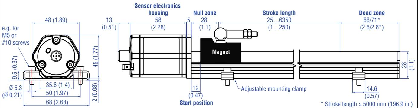
RP5-M, example: Connection type EXX/GXX/LXX/UXX (angled cable outlet)
