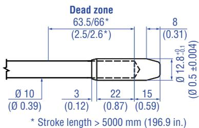
Mechanical option »M«: Thread M4 at rod end for threaded flange M18×1.5-6g or ¾"-16 UNF-3A
