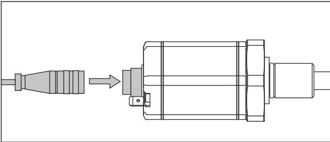
Fig. 85: Connection of adapter cable to R-Series V sensor with connector outlet
