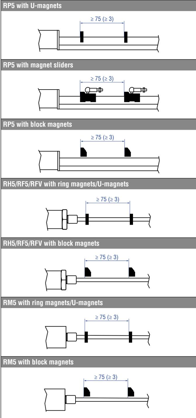
Fig. 61: Minimum distance between magnets for differential/multi-position measurement (RP5, RH5, RF5, RFV, RM5)
