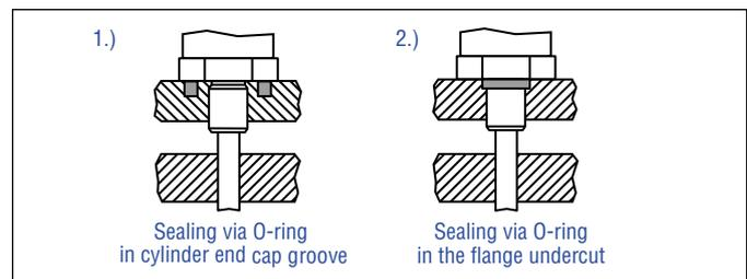
Fig. 25: Possibilities of sealing
