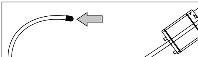
Fig. 66: Remove the transport cap from the RH5-B-F before installation
