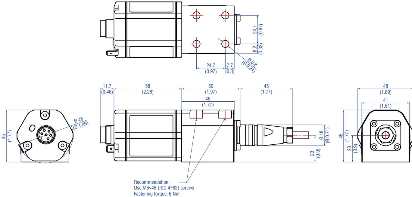
Controlling design dimensions are in millimeters and measurements in ( ) are in inches
