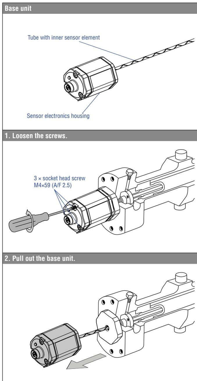
Fig. 63: Replacement of the base unit (e.g. RH5 sensor), part 1
