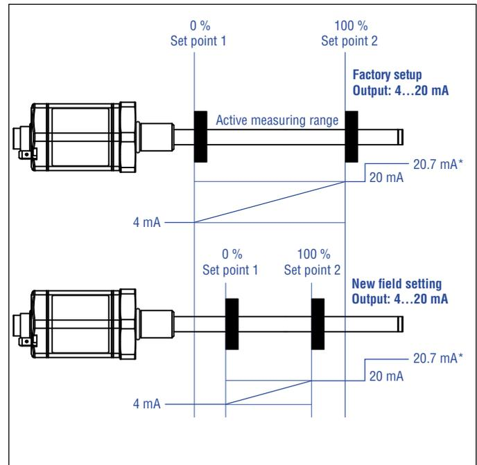
Fig. 82: Shifting the start position (set point 1) and end position (set point 2)
