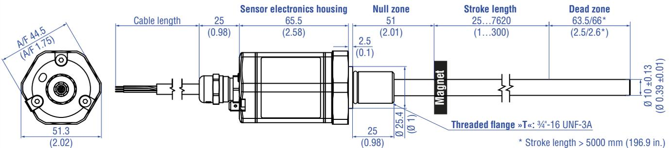
Mechanical option »B«: Bushing on rod end for threaded flange M18×1.5-6g or ¾"-16 UNF-3A
