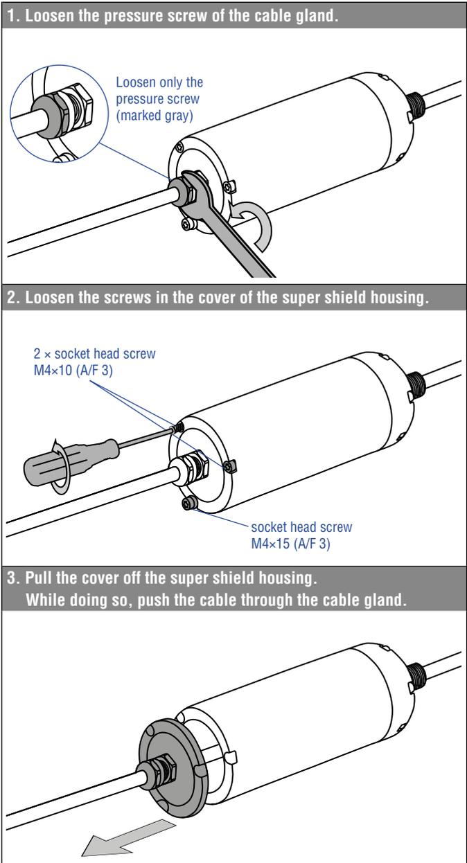
Fig. 68: Replacement of the base unit on model RM5, part 1
