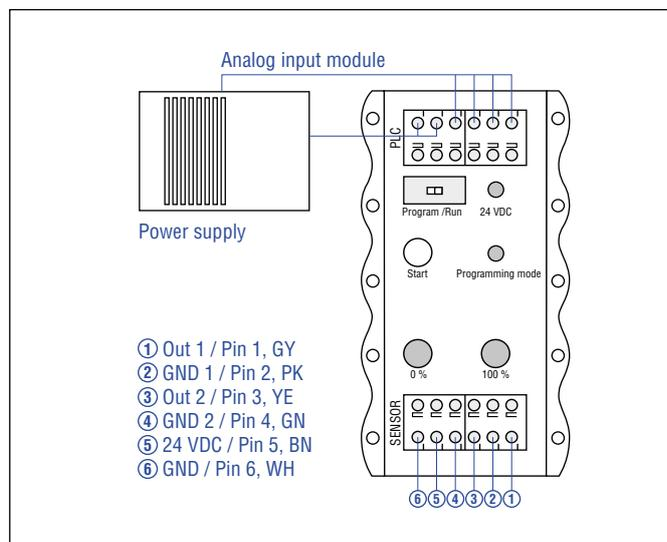
Fig. 105: Connect cabinet programmer
