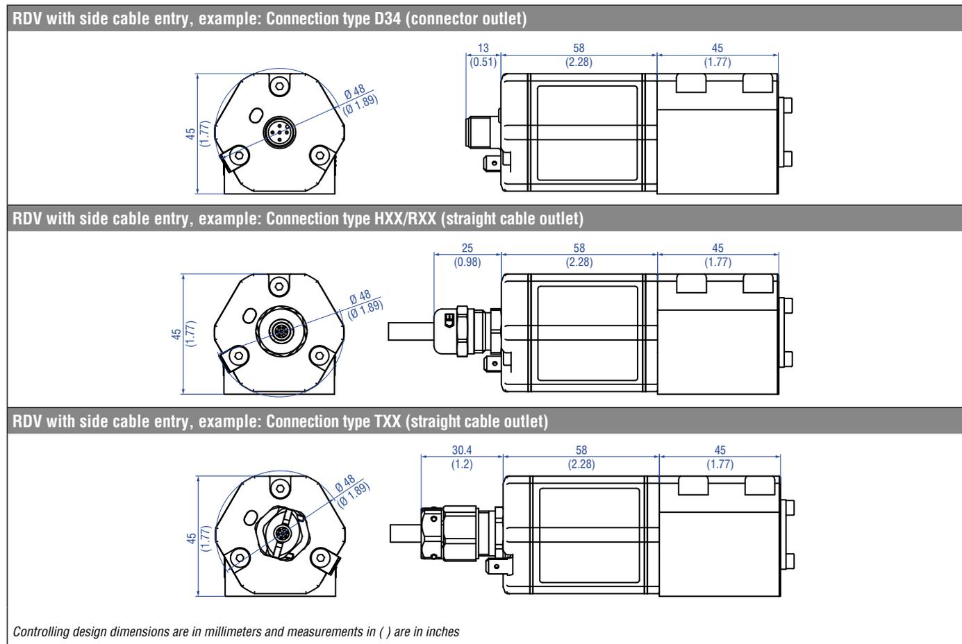
Fig. 38: Temposonics® RDV sensor electronics housing, part 2
