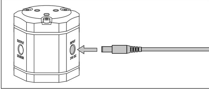
Fig. 88: Connection of power supply to the TempoLink® smart assistant
