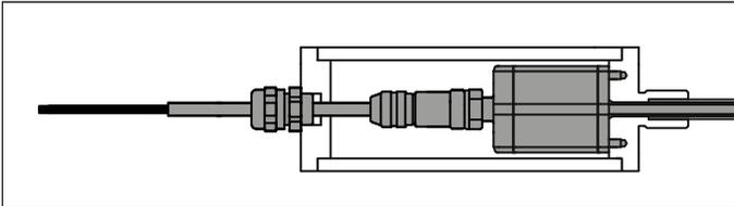
Fig. 67: Base unit in the super shield housing of the RM5
