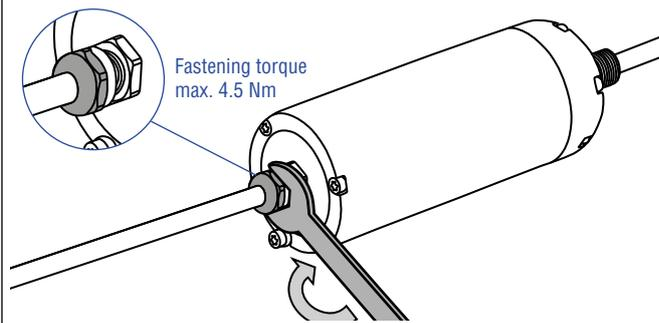
Fig. 71: Replacement of the base unit on model RM5, part 4
