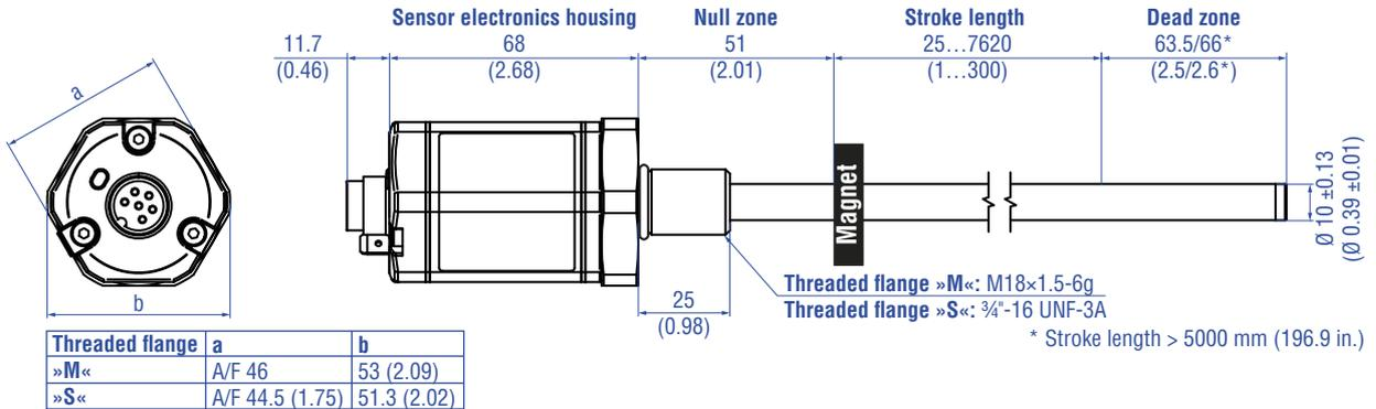
RH5-T-A/F/V – RH5 with threaded flange ¾"-16 UNF-3A with raised-face, example: Connection type EXX/GXX/LXX/UXX (angled cable outlet)
