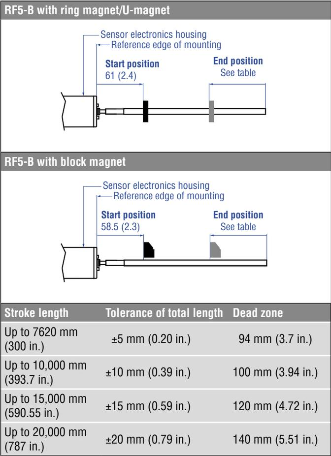
Fig. 56: Start- and end positions of magnets for RF5
