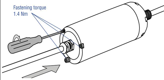
Fig. 70: Replacement of the base unit on model RM5, part 3
