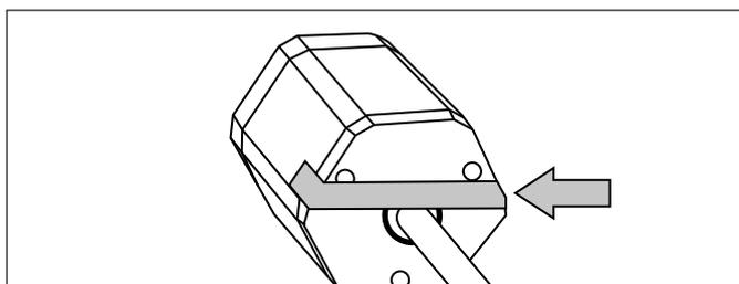
Fig. 65: Remove adhesive strips
