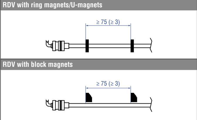
Fig. 62: Minimum distance between magnets for differential/multi-position measurement (RDV)
