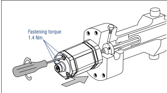
Fig. 64: Replacement of the base unit (e.g. RH5 sensor), part 2
