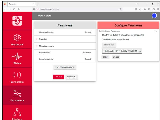
Fig. 98: Uploading a cek file to an R-Series V Analog sensor with the same stroke length
