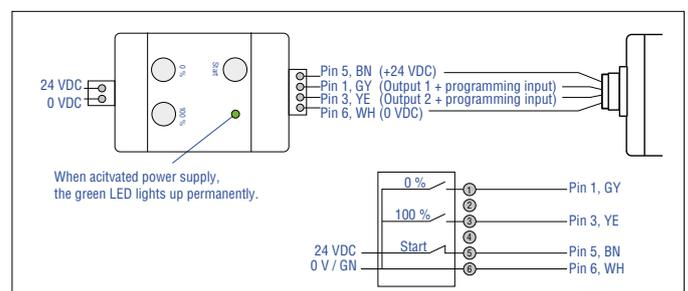
Fig. 103: Connect hand programmer
