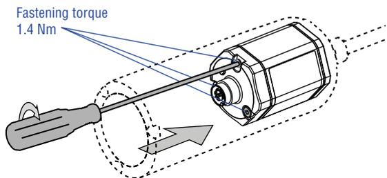
8. Attach the connector to the base unit in the super shield housing.
