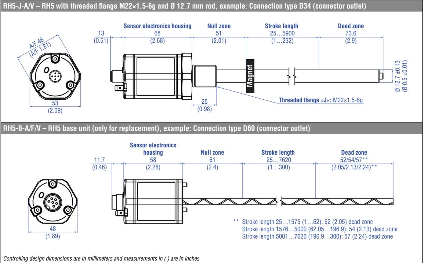
Fig. 7: Temposonics® RH5 with ring magnet, part 2
