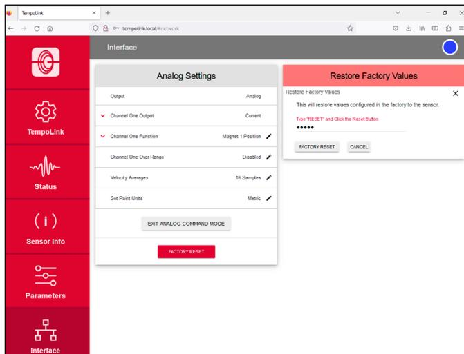
Fig. 101: Reset sensor to factory settings
