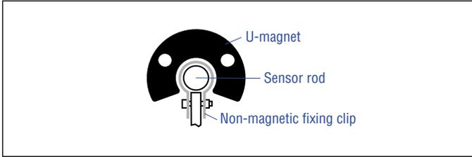
Fig. 52: Example of sensor support (part no. 561 481)
