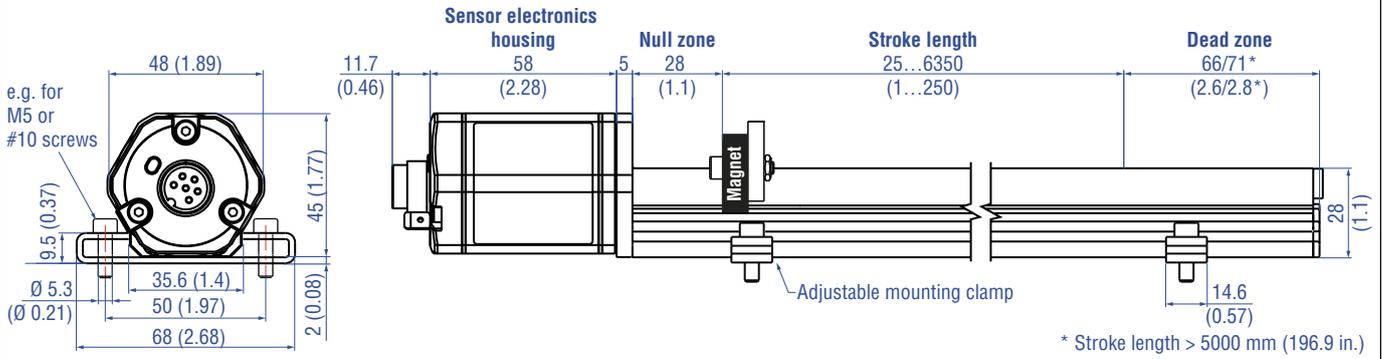
RP5-G/S, example: Connection type D34 (connector outlet)
