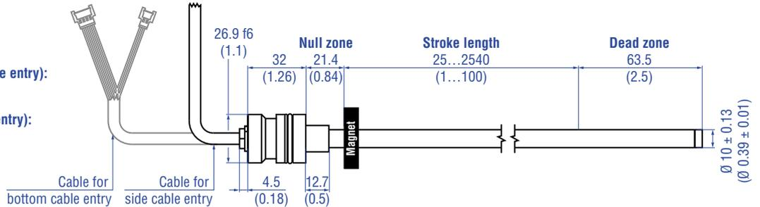
Controlling design dimensions are in millimeters and measurements in ( ) are in inches
