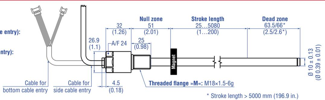
**Threaded flange »T« (for bottom or side cable entry)**
