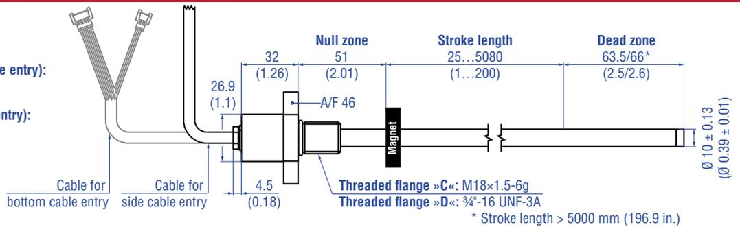
**Threaded flange »M« (for bottom or side cable entry)**
