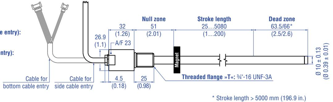
**Pressure fit flange »S« (for bottom or side cable entry)**
