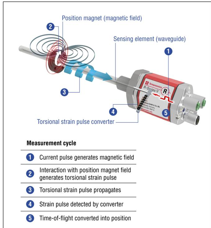
Fig. 1: Time-of-flight based magnetostrictive position sensing principle
