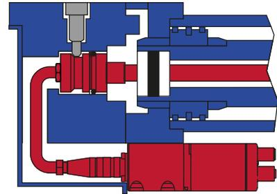
**RDV with side cable entry, example: Connector D58 (connector outlet)**
