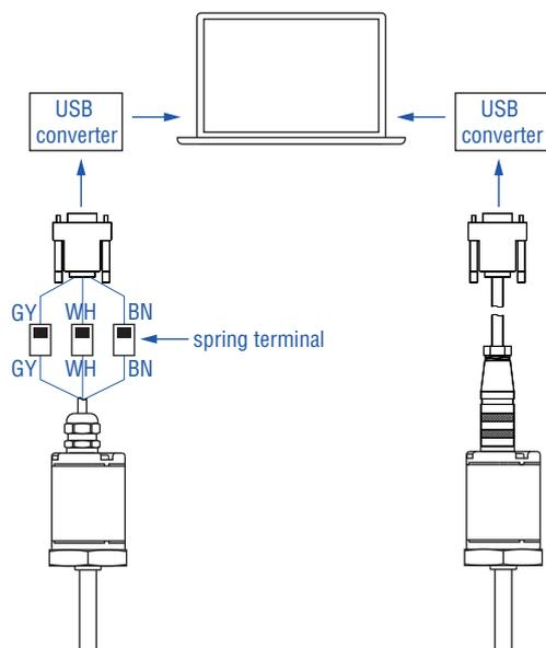
Fig. 26: Programmer connection (left: with spring terminal, right: with cable)
