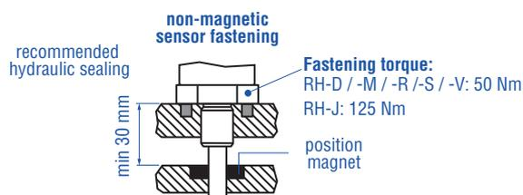
Fig. 14: Installation with non-magnetizable material
