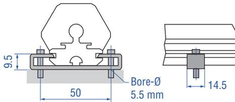
Fig. 8<sup>7</sup>: Mounting clamps with cylinder screw M5 × 20, fastening torque < 5 Nm
