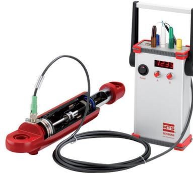
MH-Series Analog/PWM Tester, part no.: 280618
