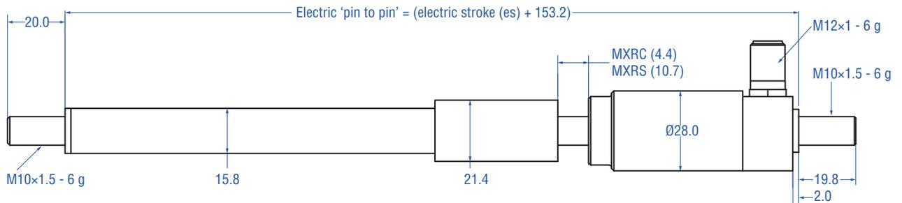
Figure 1. MH-Series Model MXR sensor dimension reference (Model MXRS shown)
