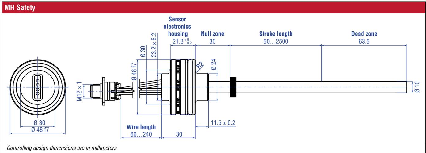
Fig. 3: Temposonics® MH Safety with ring magnet
