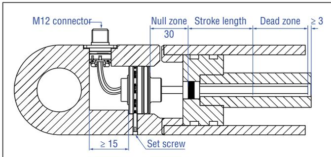
Fig. 7: Example of In-Cylinder assembly
