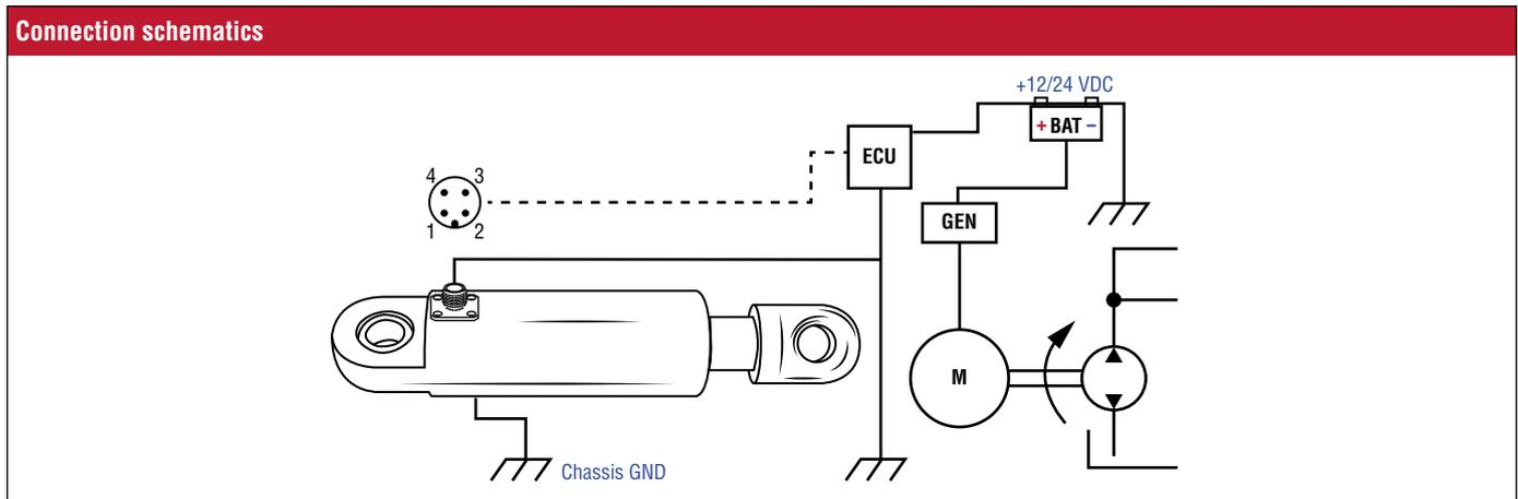
Fig. 6: Connection schematics
