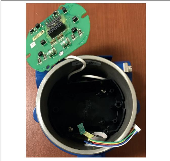
Fig. 6: Sensing element Disconnected
