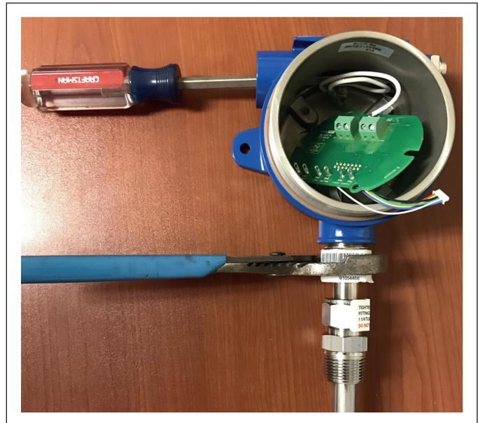
Fig. 8: Housing removal
