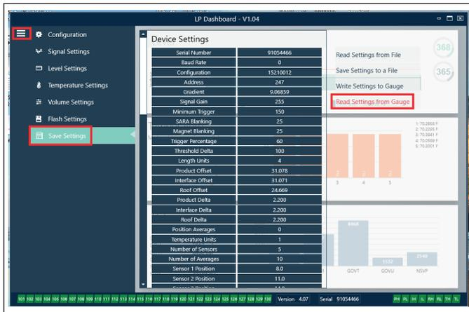
Fig. 18: LP dashboard - save settings - read from gauge
