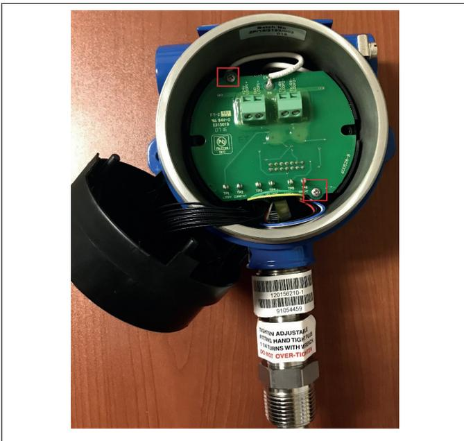
Fig. 3: Screw removal
