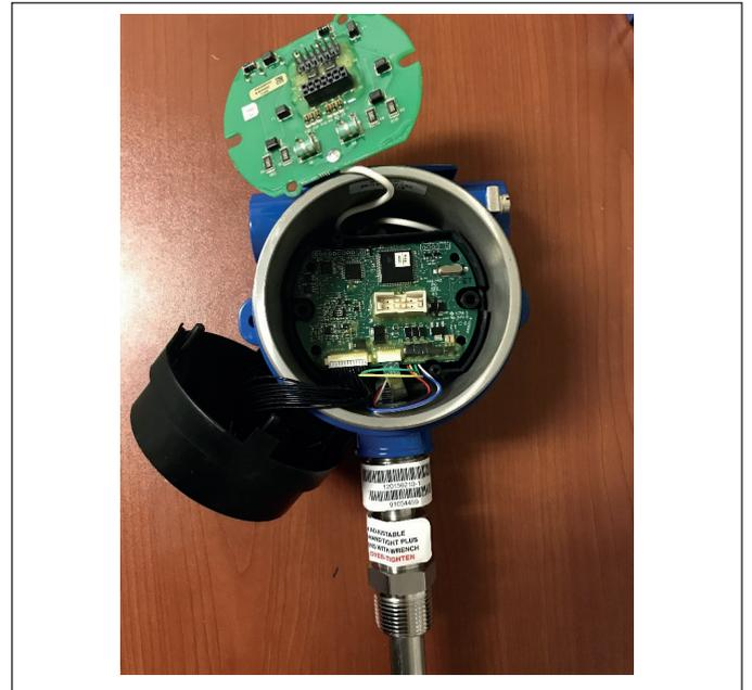
Fig. 4: Top board removed
