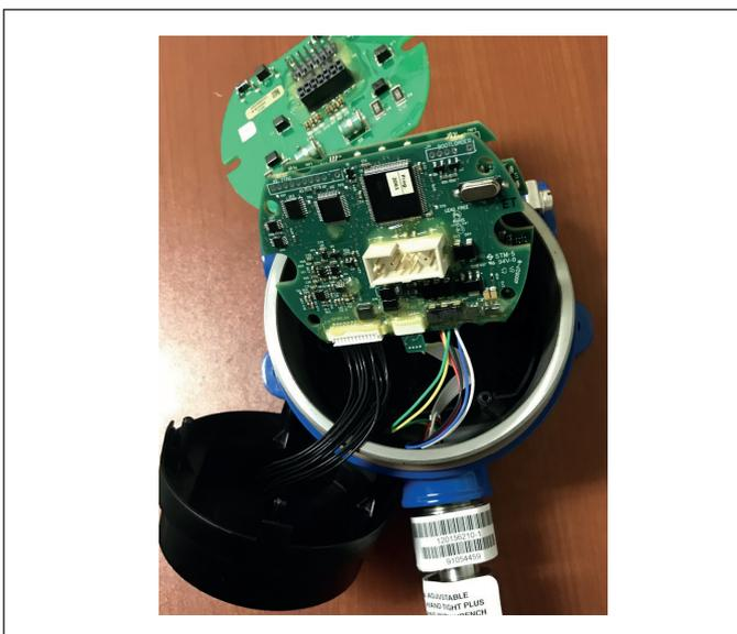
Fig. 12: All boards removed
