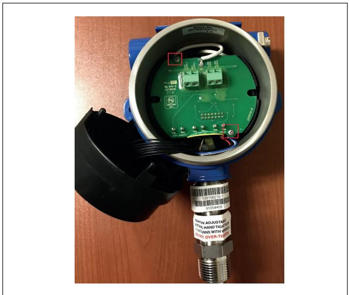
Fig. 10: Screw removal
