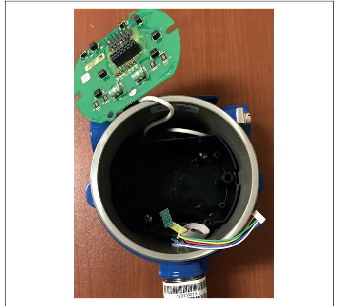
Fig. 13: Sensing Element disconnected
