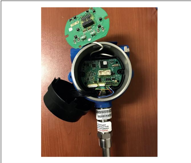
Fig. 11: Top Board Removed
