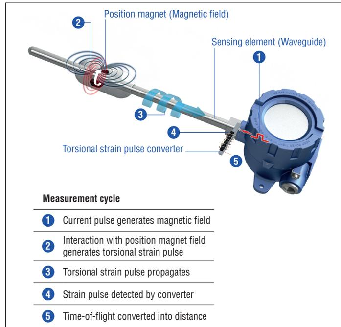
Fig. 1: Time-of-flight based magnetostrictive position sensing principle
