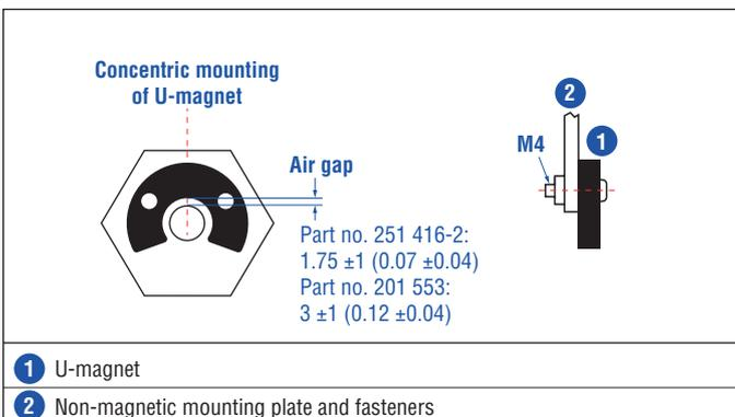
Fig. 10: Mounting of U-magnet (part no. 251 416-2)
