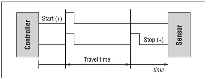
Fig. 17: Functional diagram of sensor with Start/Stop interface
