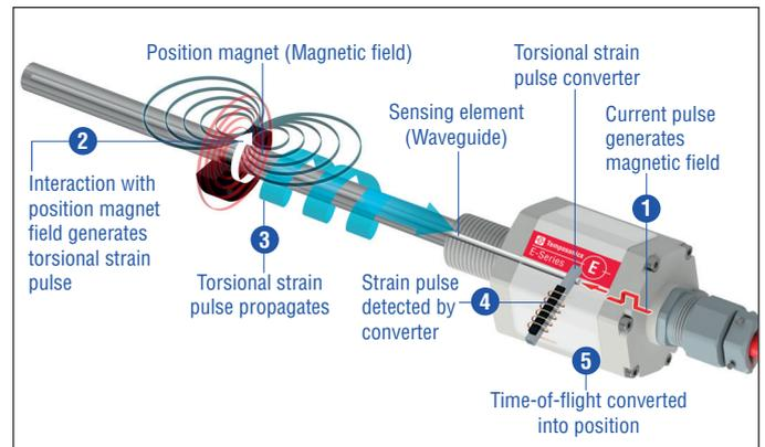
Fig. 3: Time-of-flight based magnetostrictive position sensing principle
