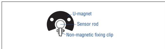
Fig. 12: Example of sensor support (part no. 561 481)
