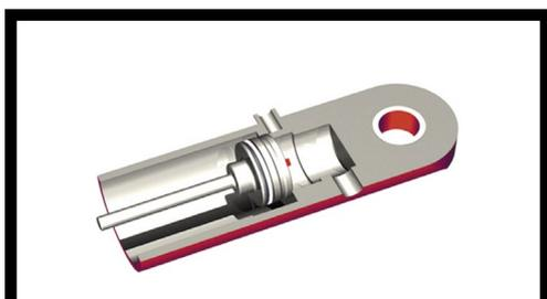
2 Slide the sensor carefully into the seat. Pay attention to connecting wires and cables.
