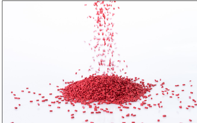
Fig. 2: Plastic granulate for injection molding or extrusion
